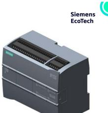
SIMATIC S7-1200, CPU 1215C, compact CPU, AC/DC/relay, 2 PROFINET ports, onboard I/O: 14 DI 24 V DC; 10 DO relay 2 A, 2 AI 0-10 V DC, 2 AO 0-20 mA DC, power supply: AC 85-264 V AC at 47-63 Hz, program/data memory 200 KB
