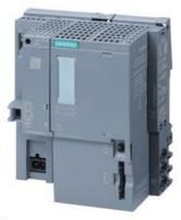
SIMATIC DP, CPU 1512SP-1 PN for ET 200SP, central processing unit with work memory 400 KB for program and 2 MB for data, 1st interface: PROFINET IRT with 3-port switch, 6 ns bit performance, SIMATIC Memory Card required, BusAdapter required for port 1 and 2
